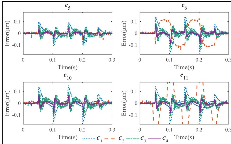
**Figure 12.** Track errors at the 5<sup>th</sup>, 6<sup>th</sup>, 10<sup>th</sup> and 11<sup>th</sup> iteration respectively.
