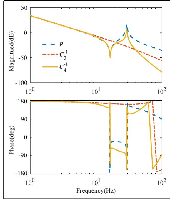
Figure 5. Bode diagram of nominal model and inversion of  $C_3, C_4$  at the 10<sup>th</sup> iteration in simulations.
