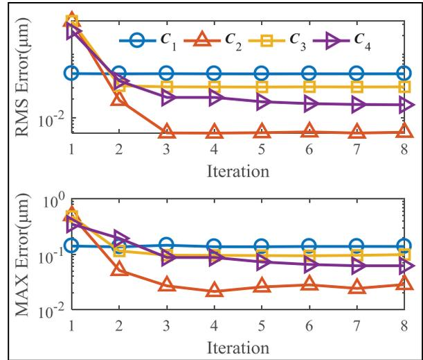
**Figure 9.** RMS and MAX errors of fixed reference tracking.
