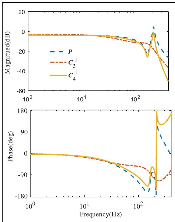
**Figure 13.** Bode diagram of nominal model and inversion of  $C_3$ ,  $C_4$  at the 15<sup>th</sup> iteration in experiments.
