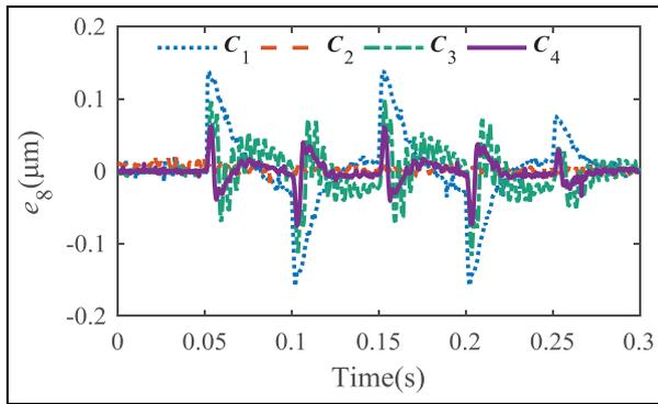
Figure 10. Tracking errors of fixed reference at the 8<sup>th</sup> iteration.
